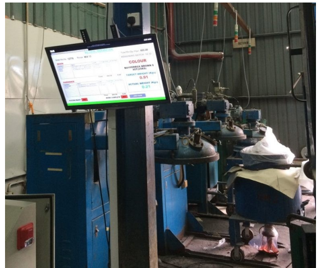
Mixer automation system screen used by operators during material preparation
