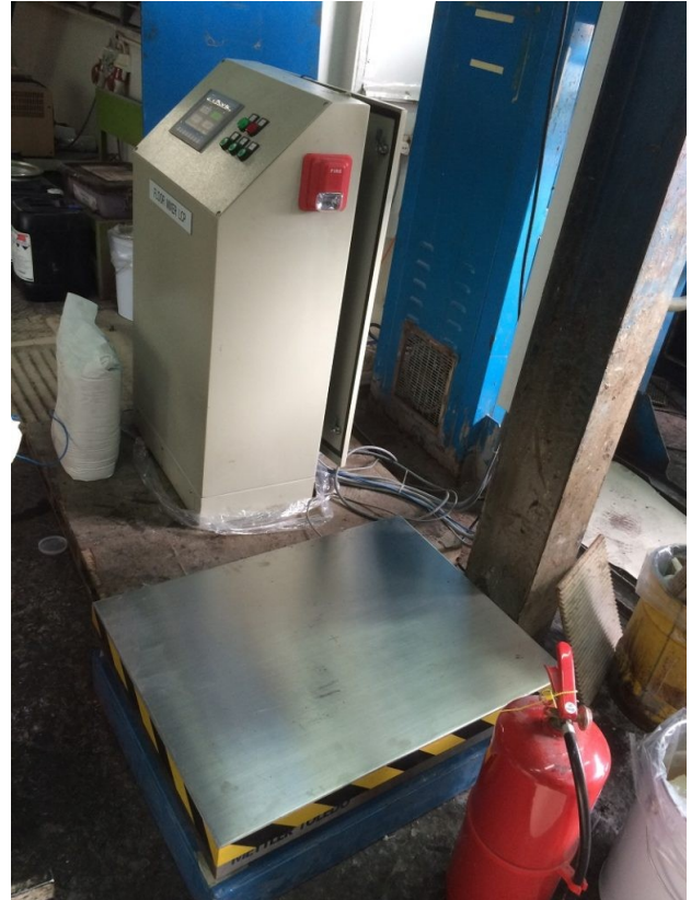
Digital weighing scale is one of the instruments involved in the mixer automation for material preparation
